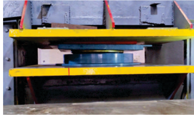
Photo-66 Rotation Test on Spherical Bearing.
